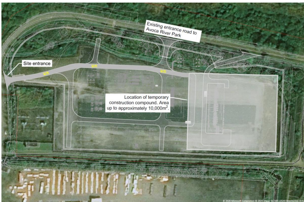
Figure 6.9: Indicative Substation Construction Compound Stage 2
